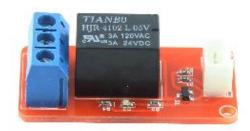
The Crowtail- Relay module is a digital normally-open switch. Through it, you can control circuit with high voltage/ larger current, with low voltage, say the 5V logic of Arduino board.
