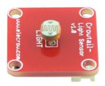
The Crowtail- Light Sensor module incorporates a light dependent resistor (LDR) to detect the lightness. Typically, the resistance of the LDR will decrease when the ambient light intensity increase, it means that the output signal from this module will be higher in bright light, and lower in the dark.
