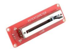
The Crowtail- Linear Potentiometer module incorporates a linear variable resistor with a maximum resistance of  $10K\Omega$ . When you move the slider from one side to the other, its output voltage range from 0 V to the VCC you applied.
