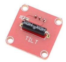
The Crowtail- Tilt Switch is a sensor to detect the station of forwards. It outputs logic LOW in Horizontal direction and logic HIGH in Vertical direction.
