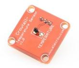
The Crowtail- Thermistor Temperature Sensor uses a thermistor to detect the ambient temperature.
